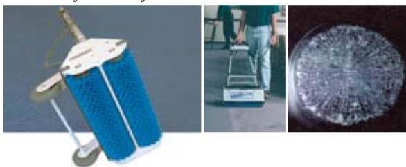
the sticky and oily residue that attracts soil on contact. The GLS machine works the Crystal Dry deep into the pile and loosens foreign solid materials, lifting the carpet pile at the same time. As the Crystal Dry chemicals dries, it encapsulates the soil in crystals that are then dry extracted by vacuum. The entire interim cleaning process is pictured below
